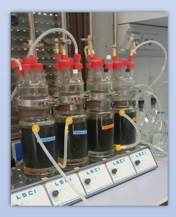
experiments The were conducted in 1 liter reactors (Figure 1) with a mixture substrate/inoculum 1:1, (in VS proportions).
